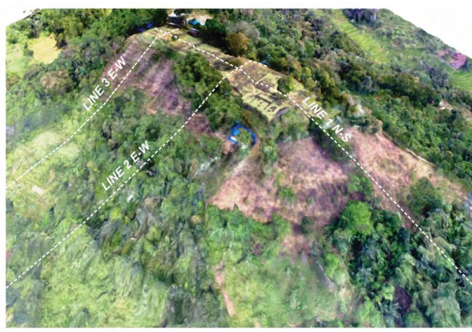
Sup.Figure.G.2. Index map showing the survey lines for the seismic tomography survey.
