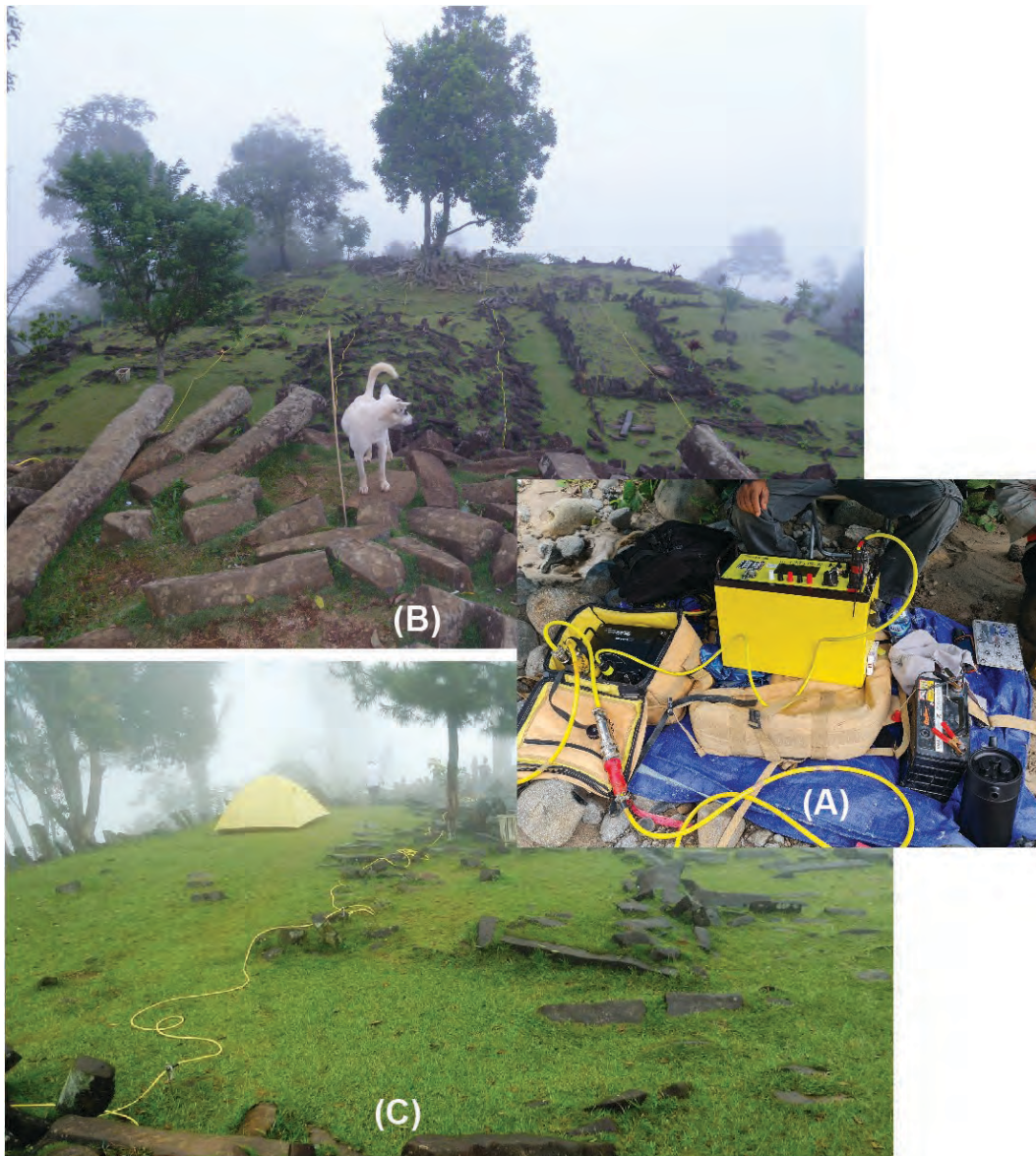
Sup.Figure-F.1. displays the ERT survey conducted using the SuperSting R8 system. (A) The main units of the SuperSting R8 system, along with the switchbox and battery used for powering the survey equipment. (B) The cables utilized for the 3D survey are shown, spread out in four lines. This configuration allowed for comprehensive data collection and imaging of the subsurface. (C) In the 2D survey setup, a cable line with specific spacing is depicted, along with electrode poles positioned at regular intervals.
