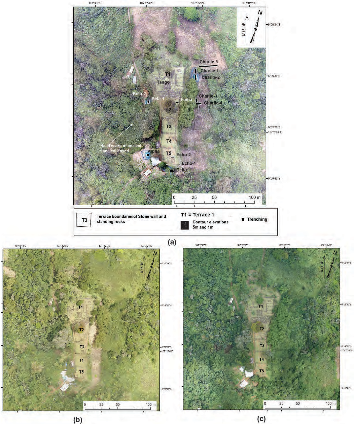
Sup. Figure A.3. Thematic Maps: (a) The Orthophoto developed from the drone survey in 2014 in collaboration with the Photographic Team of the University of Pasundan, Bandung, West Java. Contour elevations are from the geodetic survey; (b) Drone Orthophoto developed the Aero Geosurvey Surveying Co in 2019; (c) Orthophoto map, developed from by Zona Spasial Co in 2020.
