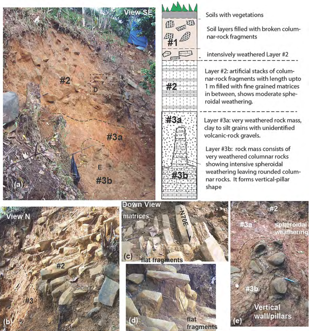
FIGURE 3 Beta-2 cliff exposures on the west slope. (a) Field photo and interpreted stratigraphy of the subsurface layers. (b) Side view highlighting Unit 2 and its distinct boundary with the underlying Unit 3. (c) Plan view of Unit 2, showcasing the alignment of columnar rocks enclosed in a fine-grained mortar. (d) Photo displaying planar rock fragments inserted between columnar rocks. (e) Photo featuring a weathered vertical pillar composed of highly weathered columnar rocks surrounded by fine-grained materials. [Colour figure can be viewed at wileyonlinelibrary.com ]
